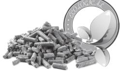
Pellets can absorb moisture after being stored in an unheated room for a long time. Ensure that the pellet container of the stove remains filled. This allows the pellets to dry properly, which results in a good start up without a lot of smoke.
