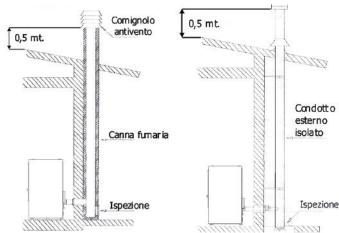
*Fig. 2: connection to the flue pipe.*
