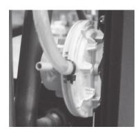
**Pressure switch:** monitors depression in the smoke duct. It is designed to shut down the pellet feed screw in the event of an obstructed flue or significant back-pressure in the presence of wind. At the time of the pressure switch will show **"ALAR-DEP-FAIL"**.
