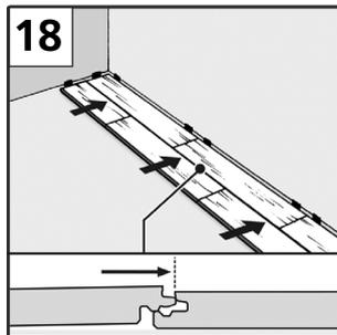
Lay out the panel piece of the second row in such a manner as to allow the panel long-sides of the 1<sup>st</sup> and 2<sup>nd</sup> row to lie parallel over one another, but not to be clicked in [16]. This means that the tongue-spring side of the first row lies on the groove side of the 1<sup>st</sup> row. Prior to clicking in place, further panels must be laid out to the end of the 2<sup>nd</sup> row. Then proceed in the same manner as for the 1<sup>st</sup> row [17, 18].
