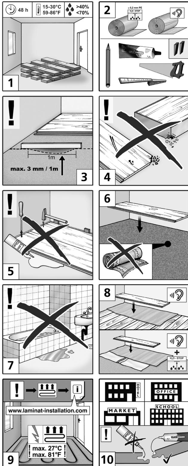
**Preparation:** Please store the packets 48 hours prior to installation under the same climatic conditions (temperature and moisture) as the actual installation process [1]. Important pre-condition for proper fitting and long-term durability of the laminated flooring is a room temperature of ca. 20°C and a relative humidity of around 50 – 70%.
