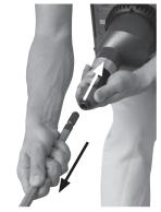
A Insert the mixing rod with HEXAFIX holder in the coupling until it snaps into place. To release the mixing rod, pull the release collar on the coupling: the mixing rod is released.
